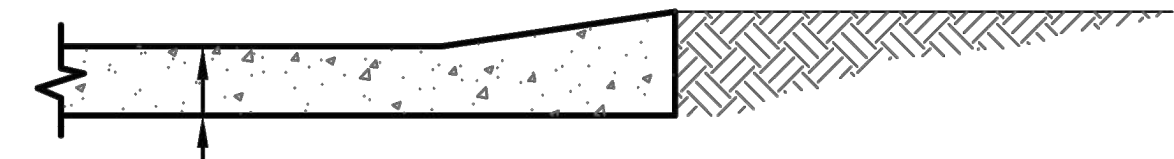
SECTION C - C T 1 =6" FOR RESIDENTIAL DRIVE APPROACH AND SIDEWALK IN DRIVE ENTRANCE
